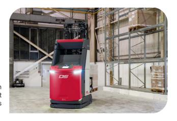
The special feature is the compact design for efficient mobility in narrow aisles from 4 m / 13.1 ft wide. The small turning radius makes ARNY particularly fast when transferring loads.
