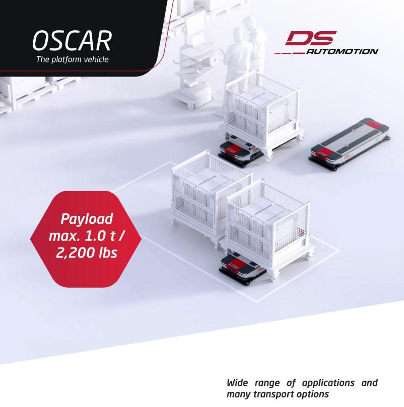
Thanks to the extremely low design, our OSCAR is suitable for a large number of undercarriage transports. Whether undercarriages, racks, boxes or roll carts, all this can be picked up, transported and set down automatically. A high payload of 1000 kg makes OSCAR an absolute transport specialist.
